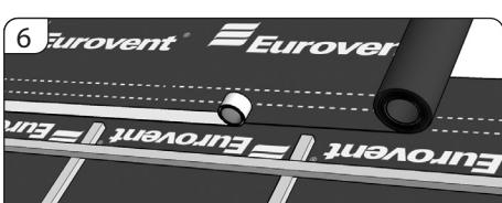
The way the roof membrane is laid as a layer of initial roof covering depends on the roof pitch and the final roof covering material. If the roof pitch is too shallow or too steep, it is recommended to read carefully the covering assembly instruction supplied by the roof covering manufacturer.
